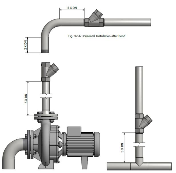
Fig. 3256 Vertical Installation after pump
